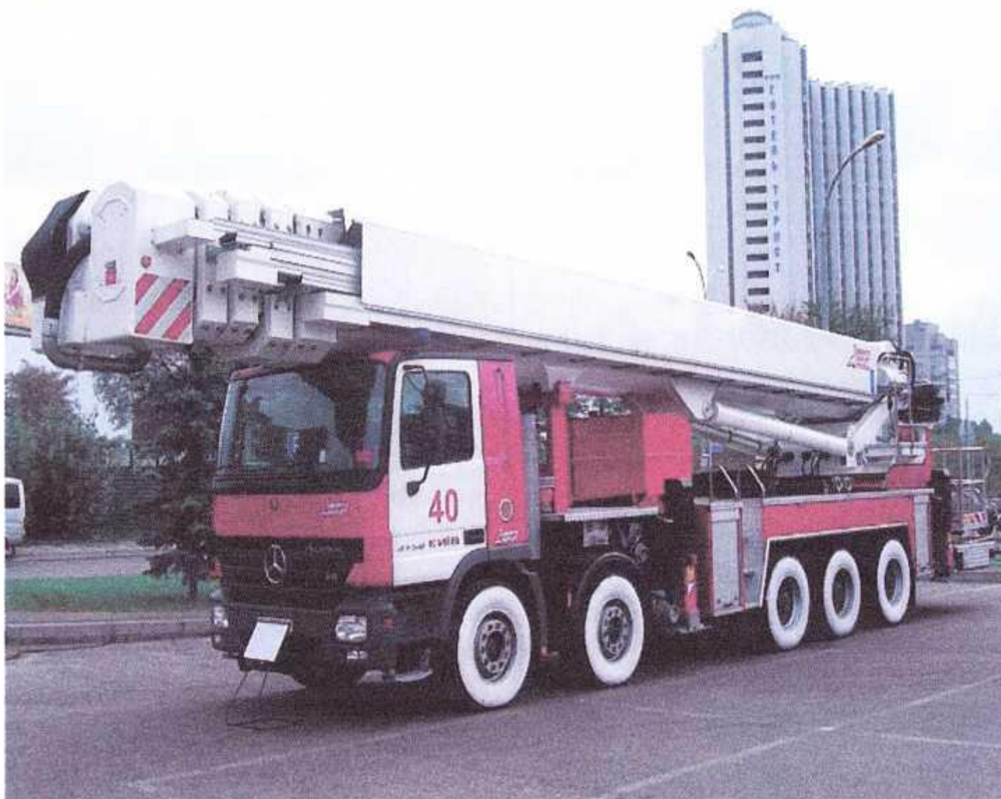
Fig.2. The most modern vehicle lift in Ukraine – Bronto Skylift F90HLA
