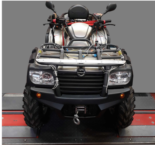
Fig. 1. Experimental off-road vehicle and the diagnostics station with mechanical vibration exciters
