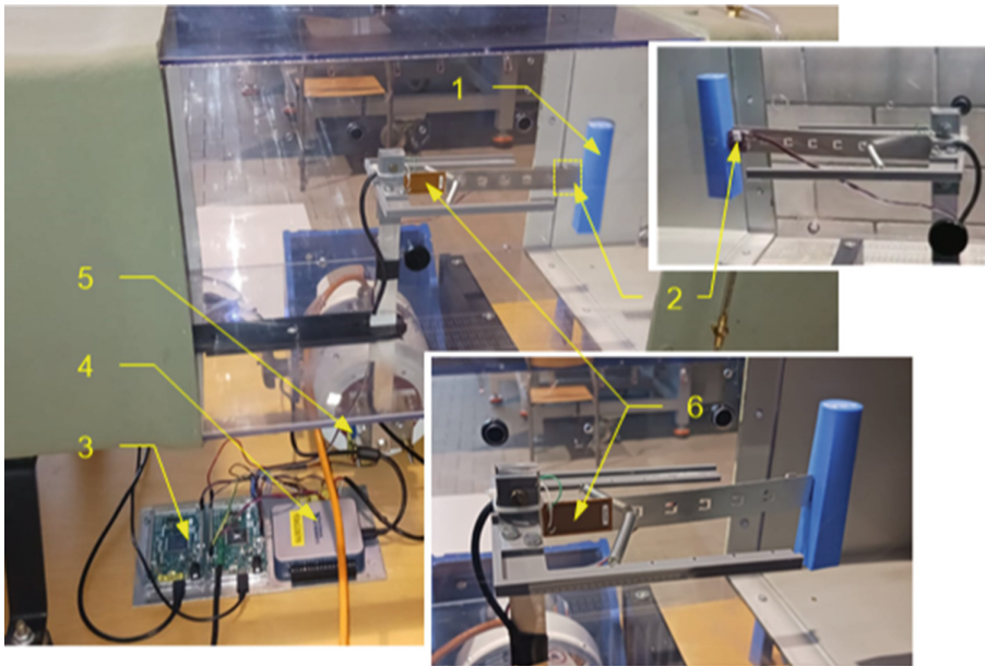
Fig. 2. The measurement section of the wind tunnel includes several components including: 1 - Bluff-body made in FDM printing technique, 2 - 3-axis MEMS digital accelerometer module at the tip of the beam, 3 - two Arduino microcontroller boards, 4 - National Instruments Data Acquisition Card, 5 - Accelerometer module mounted on the shaker plate, 6 - Piezo-patch. Full details on the elements of the test rig can be find in the reference [13].
