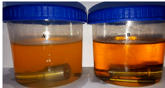
Figure 9. View of samples during the test (A) diesel fuel, (B) rapeseed oil methyl ester B100.
