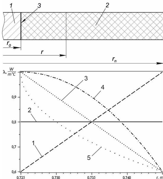
**Figure 1.** Calculation diagram of heat transfer study through friction overlays with variable thermal conductivity depending on the overlay thickness (in the radial direction) of the band-pad brake of drilling winches: 1 – pulley; 2 – overlay; 3 – friction zone.
