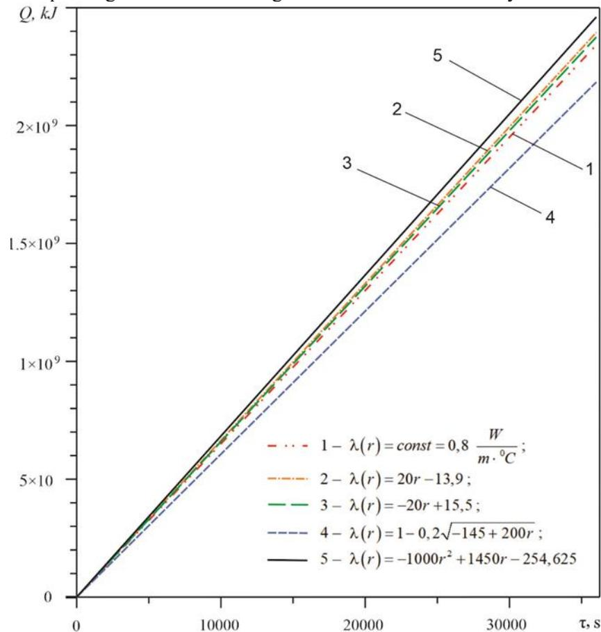
**Figure 3.** The amount of heat dissipated through the body of the friction overlay, as a function of time under different laws of the thermal conductivity coefficient change (1 – 5).
