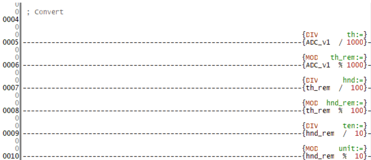
Fig. 7. Operation of converting an input number into four variables for each digit of the indicator
