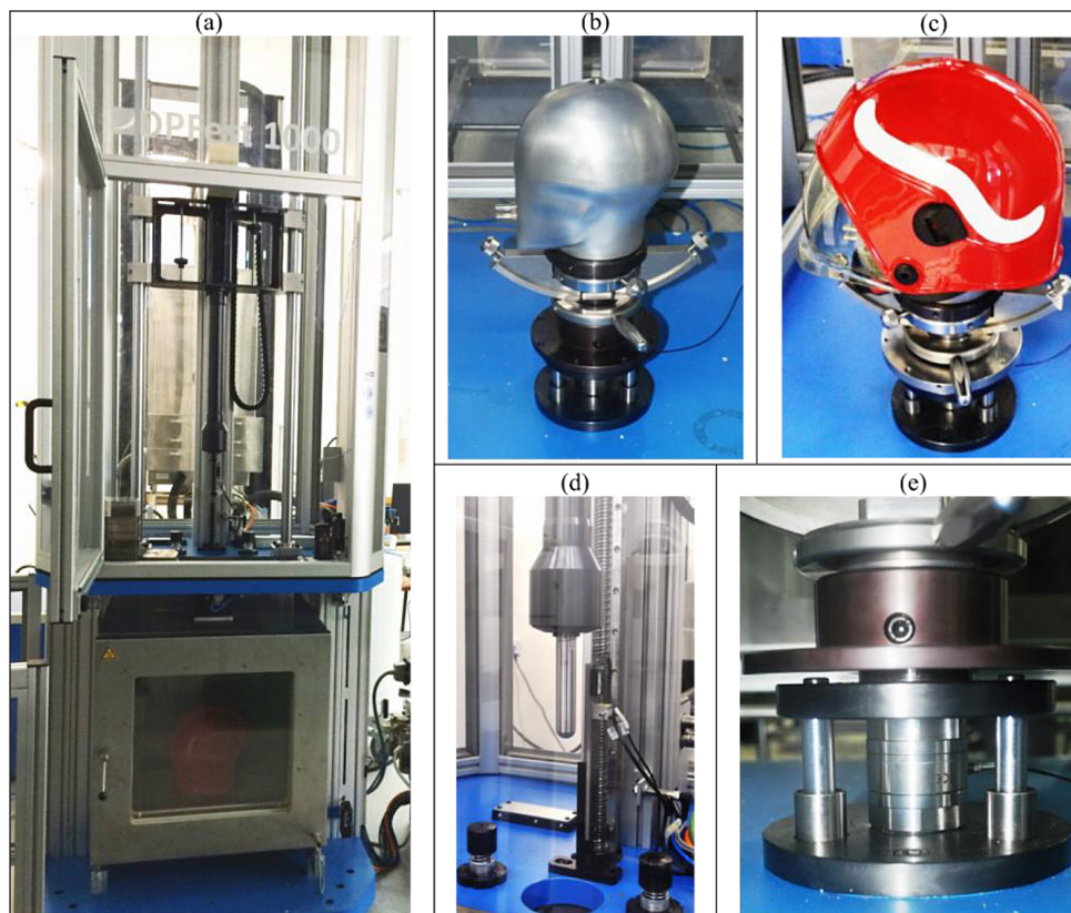
Fig. 1. Test benches for research on firefighters’ helmets under dynamic (impact) mechanical loads: a) drop hammer, b) head model, c) helmet superimposed on the head model, place of central impact marked with laser beam, d) beater, e) additional sensor under the head model, in the place of the cervical spine
