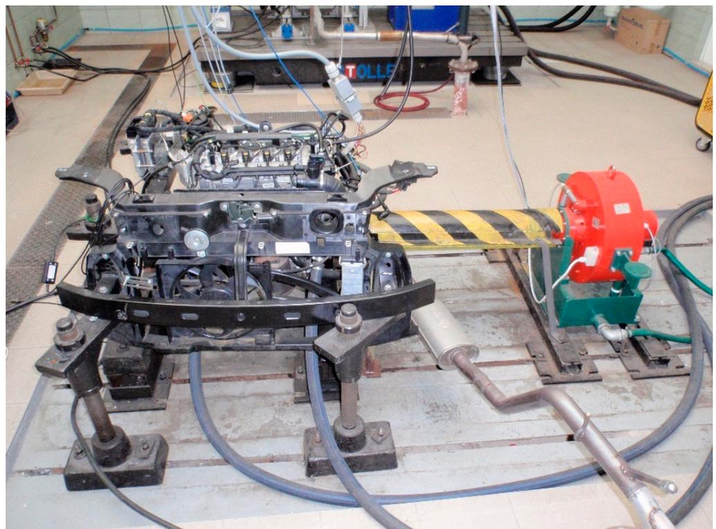
**Figure 1.** Test stand with a Fiat 1.3 JTD engine and AMX eddy current brake.
