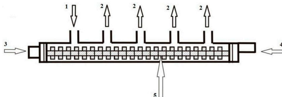
**Figure 2.** Modified high-pressure accumulator with a hydrogen reactor: 1—fuel supply, 2—fuel outlet to the system, 3—pressure sensor, 4—high-pressure regulator, and 5—hydrogen reactor.
