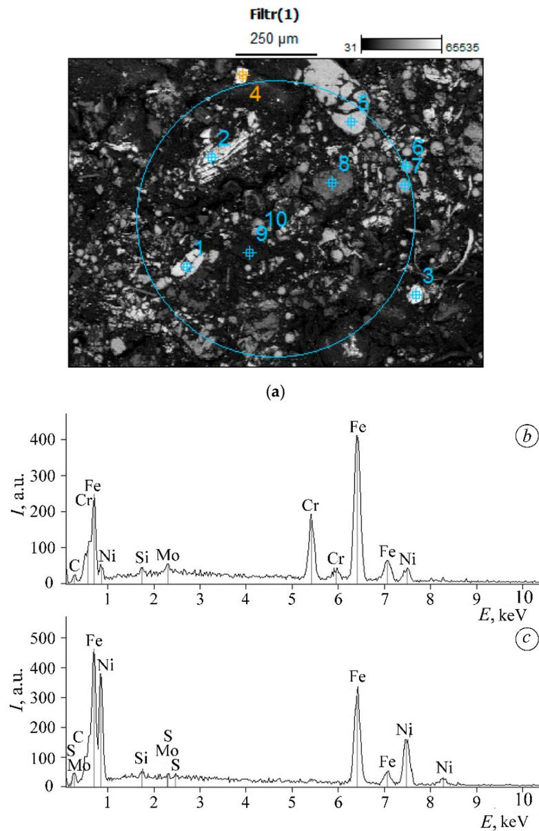
**Figure 5.** The microstructure of the wear products of the fuel injector socket as a result of the cavitation phenomenon (a) and local elemental analysis (b,c) (numbers—the points where the local elemental analysis was carried out (Table 1)).
