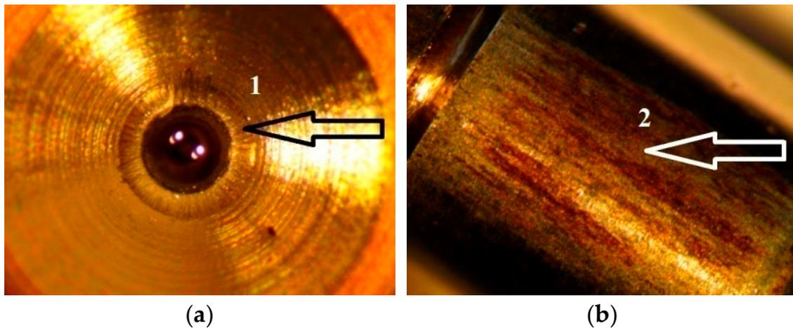
**Figure 4.** Damaged (due to cavitation) seat of the fuel injector (a) and the precision pairs of the piston of the control valve (b) (traces of cavitation, abrasive wear (1) and corrosion (2) are shown by arrows).
