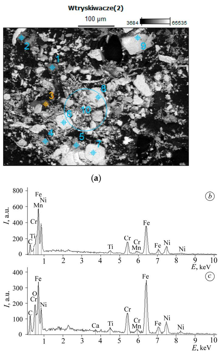
**Figure 7.** The microstructure of the wear products of the fuel injector socket as a result of the cavitation phenomenon (a) and analysis (b,c) (numbers—the points where the local elemental analysis was carried out (Table 2)).
