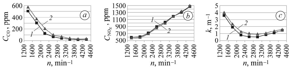
**Figure 3.** Dependence intensity of the emissions of carbon oxides CO (a) and nitrogen NO<sub>x</sub> (b) and their smokiness (c) of exhaust gases, determined by the absorption coefficient of infrared radiation  $k$  on engine revolutions, where cases of healthy (2) and damaged (1) fuel injectors.
