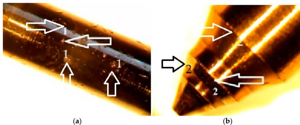
**Figure 6.** Damaged needle of the investigated fuel injector: (a) metallic filings (1), which degrade the precision pairs of the atomizer, (b) the needle damaged due to contamination, the places marked with arrows show the degraded precision pair of the atomizer needle (2).
