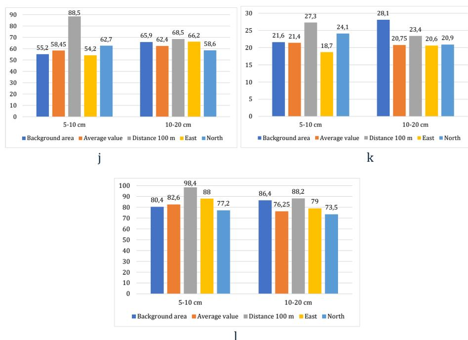
**Figure 5.** Diagrams specific mass activity of  $^{137}\text{Cs}$  - a,  $^{90}\text{Sr}$  - b,  $^{40}\text{K}$  - c in soil samples collected at 5- 10 cm and 10-20 cm horizons of the Khmelnytskyi landfill (Bq/kg).
