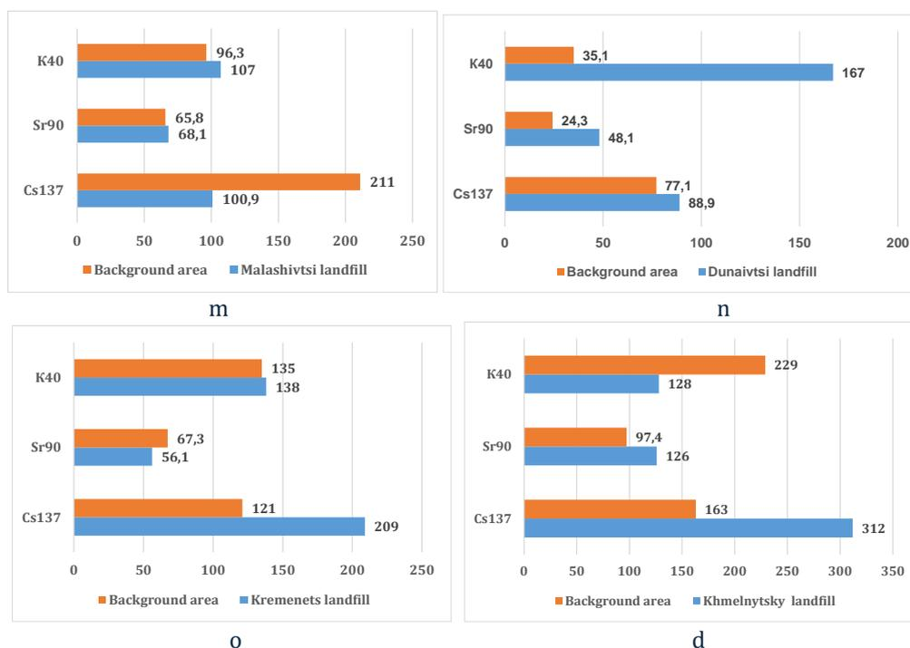
**Figure 6.** Comparative characteristics of the specific mass activity of radionuclides in plant samples collected from adjacent areas to Malashivtsi landfill - a, Dunaivtsi landfill - b, Kremenets landfill - c, and Khmelnytsky landfill - d (Bq/kg).
