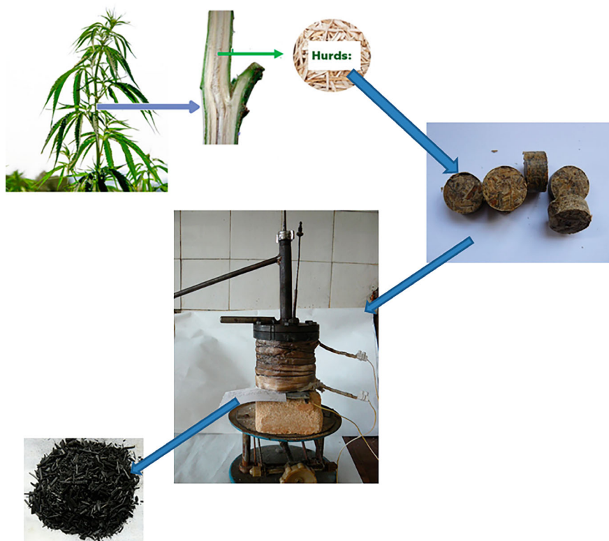
Fig. 17.1 Scheme of laboratory carbon obtaining
