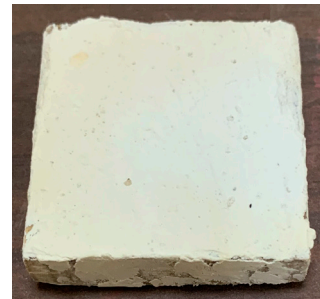
Fig. 1. Model sample of wood treated with a biocomposite coating with the addition of potassium nitrite
