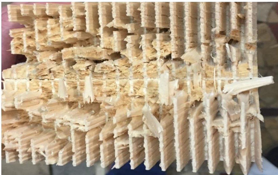
Fig. 2 – Failure pattern of specimens with imperfect adhesive application in the finger joint zone [6]
