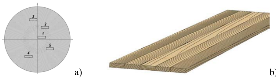
Figure 2 - a) position of the lumber in the log; b) projected view of the panel
