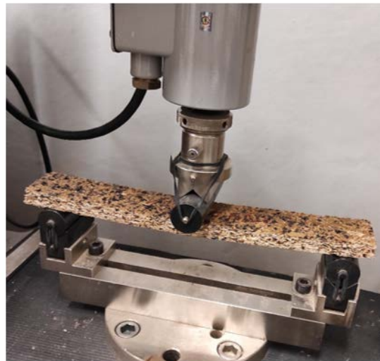
Figure 1 – The principle of BS and MOE measurement
