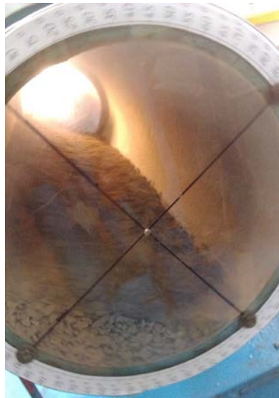
Fig.2. Material's pelletization in the rift mode
