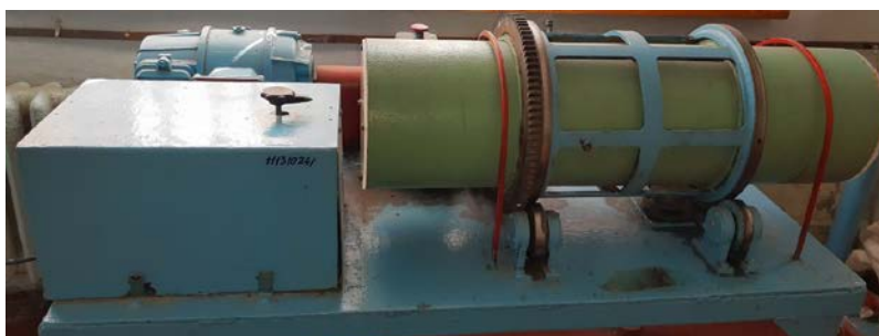
Fig.1. Drum mixer-pelletizer laboratory model
