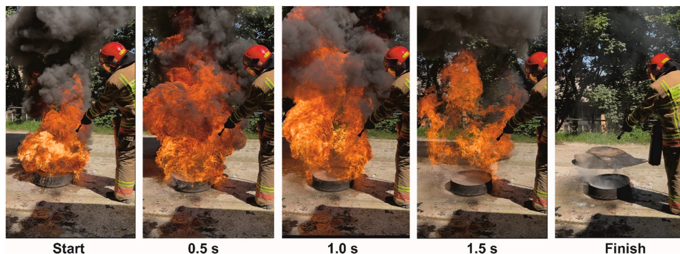
Fig. 2. Time-lapse photographic sequence of Class B fire (A-92 Euro-5 automotive petrol) suppression in an open space using misted (\text{NH}_4)_2\text{CO}_3 -based AFEA solution, illustrating the evolution from transient flare-up to complete quenching (time interval between frames: 0.5 s).
