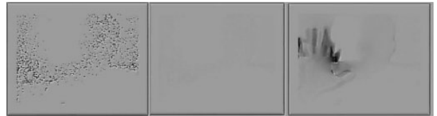
Figure 2. Real-time frame difference. From left to right: without any morphological operations, with morphological operations, example of motion.
