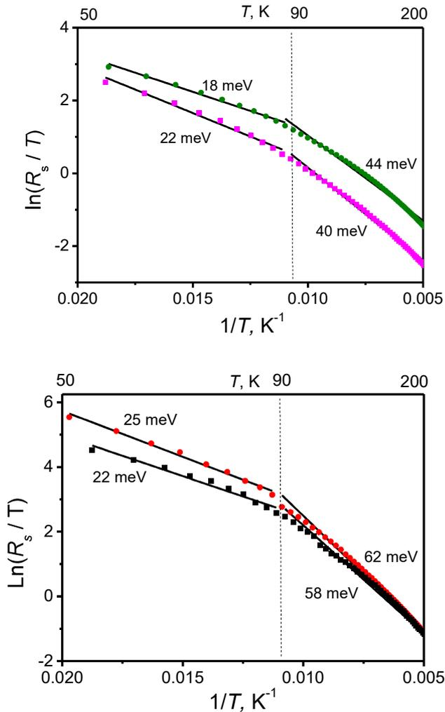
Fig. 5. Comparison of Arrhenius plots for PEDOT:PSS/MWCNT and PEDOT:PSS/SWCNT composite films. Circles denote experimental points for 12 wt% MWCNT loading; triangles denote experimental points for 16 wt% SWCNT loading. Solid lines represent linear fitting.
