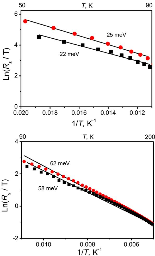
Fig. 3. Arrhenius plots for PEDOT:PSS/SWCNT composite films. Circles denote experimental points for 12 wt% SWCNT loading; squares denote experimental points for 16 wt% SWCNT loading. Solid lines represent linear fitting
