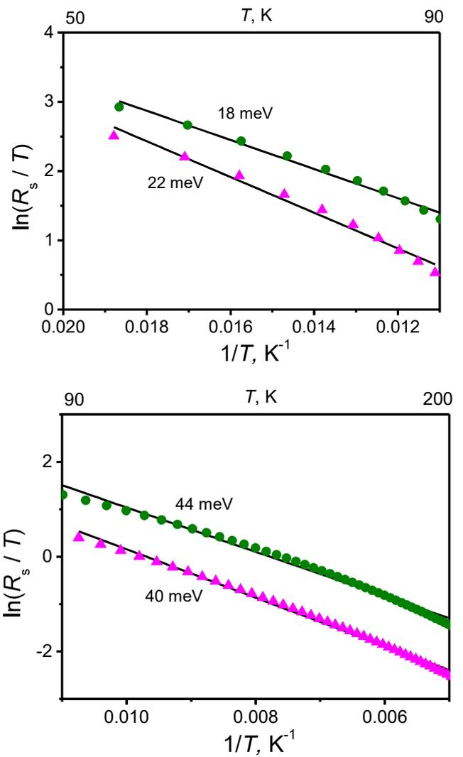
Fig. 4. Arrhenius plots for PEDOT:PSS/MWCNT composite films. Circles denote experimental points for 12 wt% MWCNT loading; triangles denote experimental points for 16 wt% SWCNT loading. Solid lines represent linear fitting.
