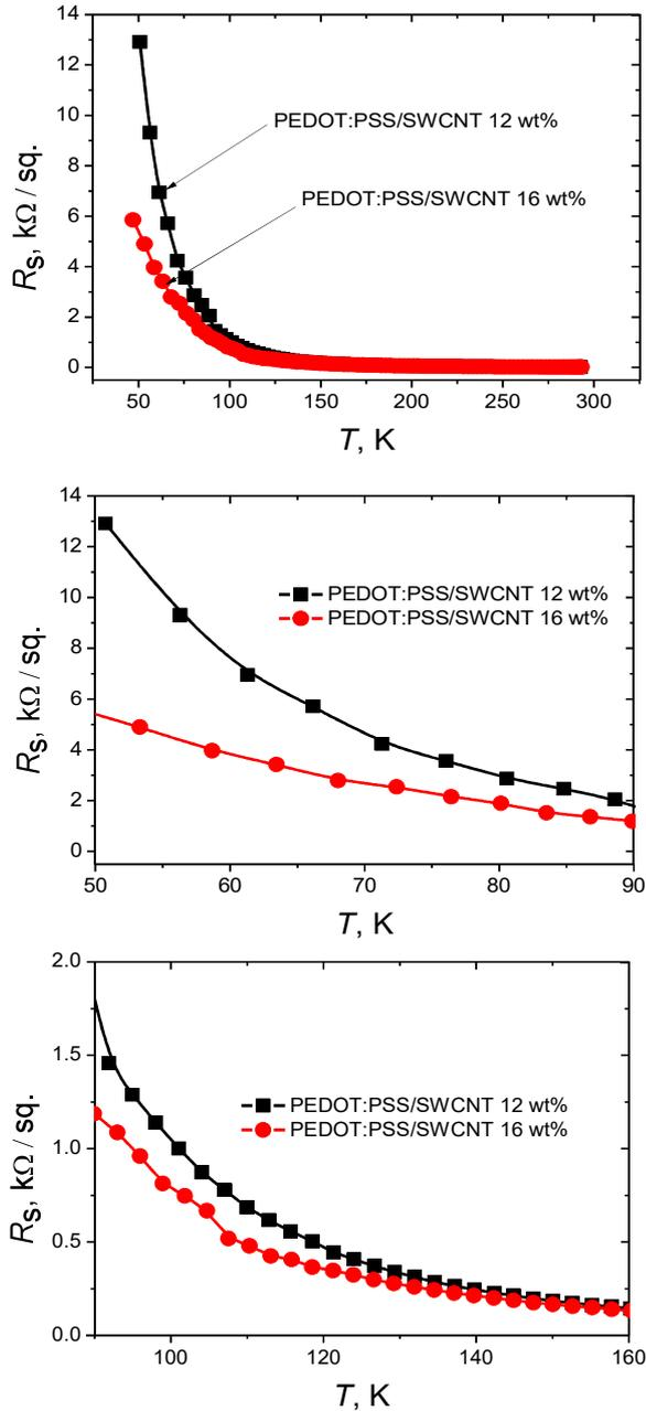
Fig. 1. Dependencies of sheet resistances on temperature for PEDOT:PSS/SWCNT composite films measured in cooling regime
