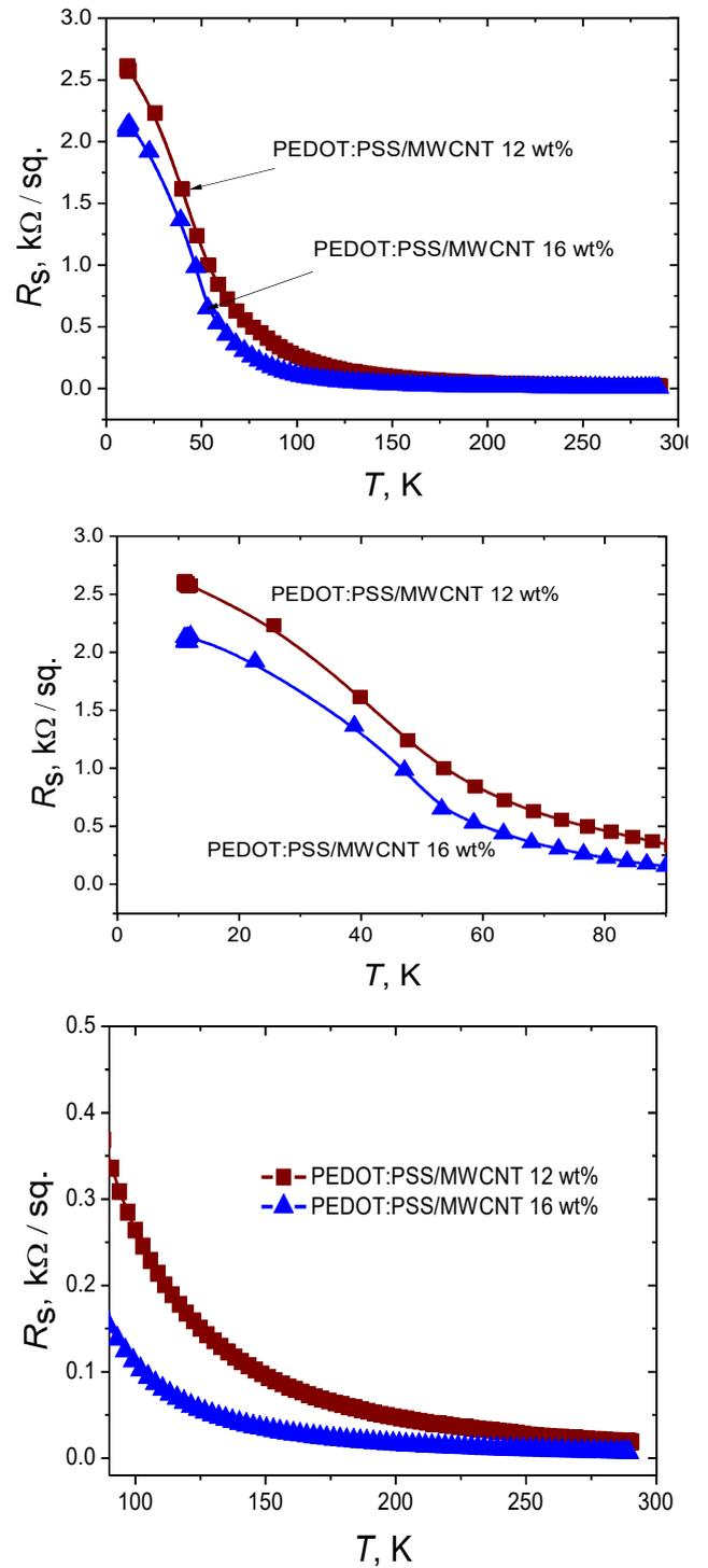
Fig. 2. Dependencies of sheet resistances on temperature for PEDOT:PSS/MWCNT composite films measured in cooling regime
