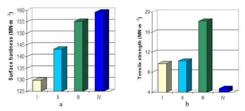
Figure 3 The surface hardness: (a) and tensile strength; (b) of the epoxy-amine composites (I – *DGEBA/PEPA*; II – *DGEBA/PEPA*-CuSO<sub>4</sub>; III – (*DGEBA/PEPA*)<sub>2</sub>-(CuOH)<sub>2</sub>CO<sub>3</sub>; IV – *DGEBA/PEPA*-CuSiF<sub>6</sub>) (SD of surface hardness and tensile strength measurements are ±5 and ±2 MN·m<sup>-2</sup>, respectively)
