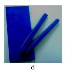
Figure 1 The samples of the epoxy-amine composites: a - DGEBA/PEPA; b - DGEBA/PEPA-CuSO<sub>4</sub>;  $c - (DGEBA/PEPA)_2$ -(CuOH) $_2$ CO<sub>3</sub>; d - DGEBA/PEPA-CuSiF $_6$
