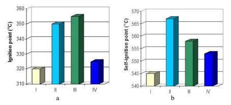
Figure 2 The ignition point: (a) and self-ignition point; (b) of the epoxy-amin composites (I – *DGEBA/PEPA*; II – *DGEBA/PEPA*-CuSO<sub>4</sub>; III – (*DGEBA/PEPA*)<sub>2</sub>-(CuOH)<sub>2</sub>CO<sub>3</sub>; IV – *DGEBA/PEPA*-CuSiF<sub>6</sub>) (SD of temperature measurement is ±1°C)
