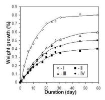
Figure 4 Water absorption of the epoxy-amine composites: I-DGEBA/PEPA; II-DGEBA/PEPA-CuSO<sub>4</sub>;  $III-(DGEBA/PEPA)_2$ -(CuOH) $_2$ CO<sub>3</sub>; IV-DGEBA/PEPA-CuSiF $_6$
