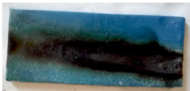
**FIGURE 3** The sample of the *DGEBA/pepa*-CuSiF<sub>6</sub>(IV) after combustibility testing [Colour figure can be viewed at [wileyonlinelibrary.com](http://wileyonlinelibrary.com)]
