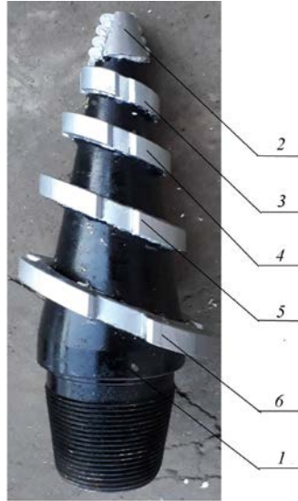
Figure 3 – Drill tool with cutting teeth of 40X structural steel. 1 - body of the drilling tool; 2 - tip equipped with carbide plates of BK8 round shape; 3,4,5,6 - cutting teeth of the boring tool
