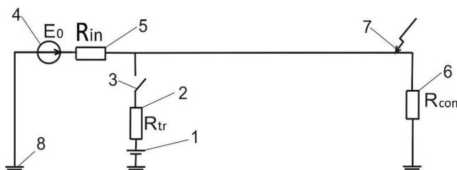
Fig. 3. Scheme of short circuit current in case of damage to the wires insulation material of the onboard mains: 1 is battery; 2 is the internal resistance of the battery; 3 is key; 4 is the electromotive force of the generator; 5 is the internal resistance of the generator; 6 is consumer resistance; 7 is the place of occurrence of the short circuit; 8 is housing.
