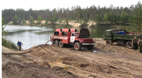
Figure 11. Application of FPS -110 (131) for extinguishing peat fires
