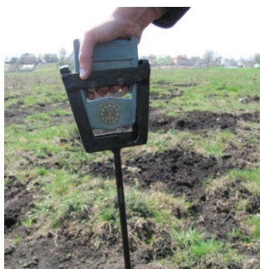
Figure 25. Determination of peat hardness (resistance) in Gamaliyivka village, Lviv region
