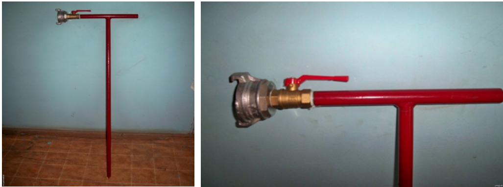
Figure 6. General view of the peat fire hose nozzles type TS-1 and TS-2
