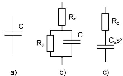
Fig. 1. Models of supercapacitors: a) ideal supercapacitor; b) equivalent supercapacitor model based on series and parallel resistances; c) equivalent supercapacitor model using fractional calculus
