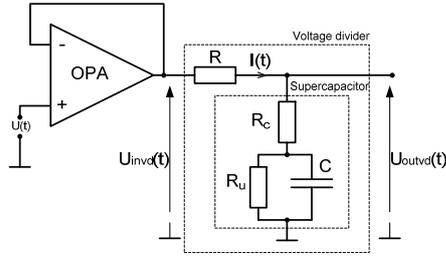
Fig. 2. The scheme used in experiments with supercapacitors
