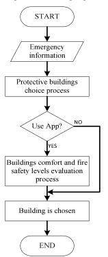
Fig. 6. The flowchart of protective building choosing process
