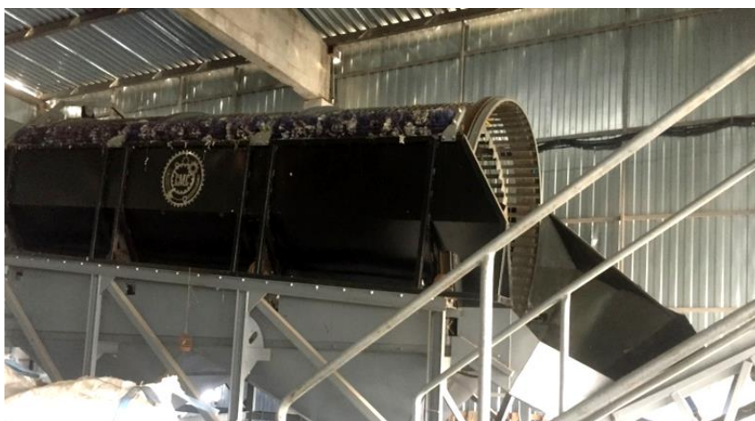
Fig.3 The waste sorting line on the landfill in Dunaivtsi (photo by Skyba T., 2020)
