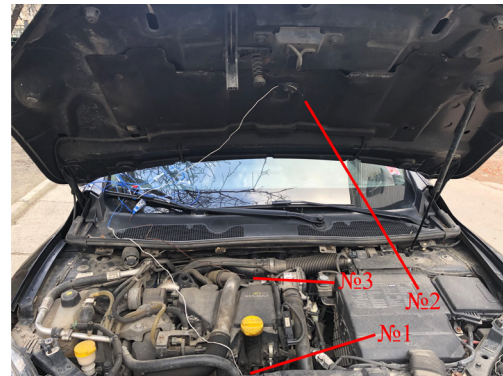
Fig. 1. Arrangement of three thermocouples in the engine compartment
