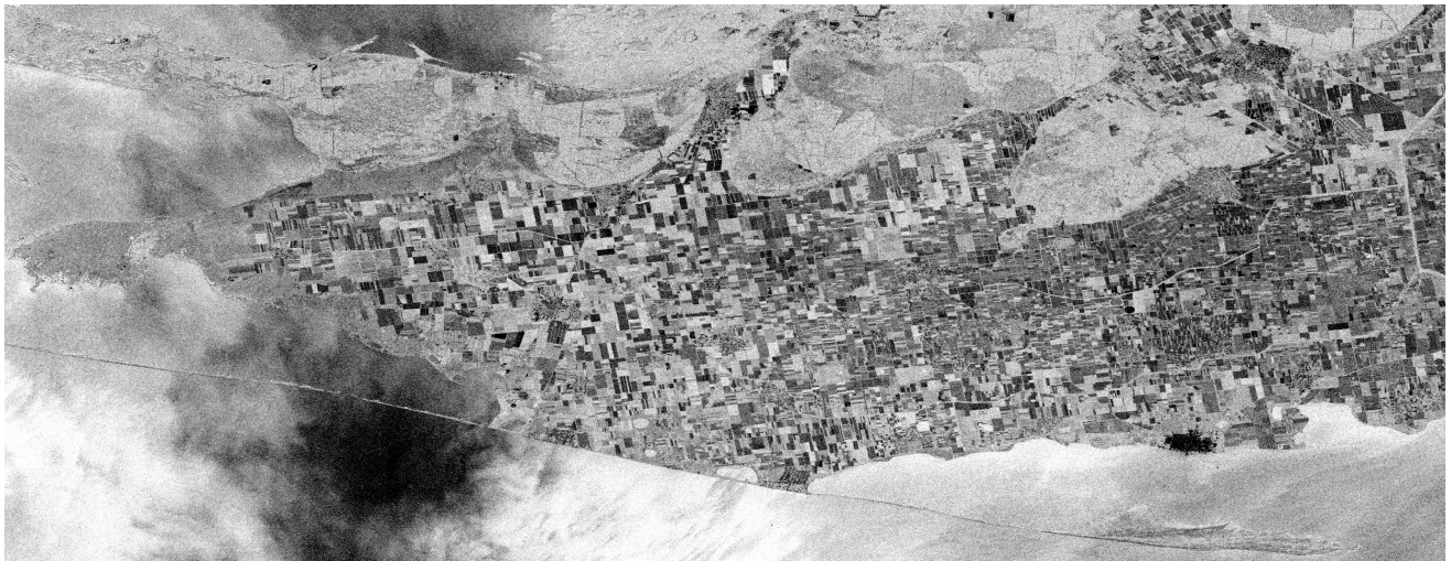
The land surface dielectric permittivity map obtained based on the Sentinel-1 dual-polarization radar image Ochakovske – Skadovsk (Ukraine), April 12, 2021, 10 m spatial resolution
