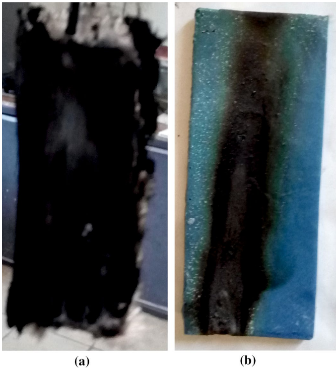
Fig. 9 The samples of EAP (a) and EA–CuSiF 6 (66) (b) after combustibility testing
