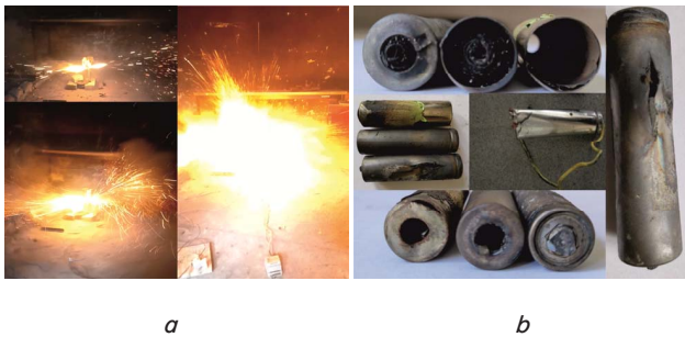
Fig. 3. Results of experimental studies to determine the critical indicators of Panasonic NCR18650B exposed to excess currents: a – the direct process of conducting experimental research; b – Panasonic NCR18650B after experimental research
