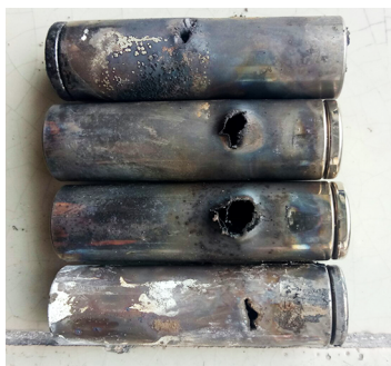
Fig. 8. LIB after conducting the experimental studies
