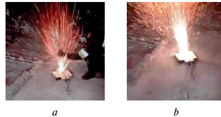
Fig. 2. The process of penetrating LIB by nail
