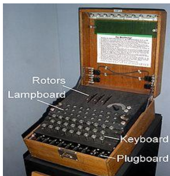
Fig. 11. The Enigma machine
