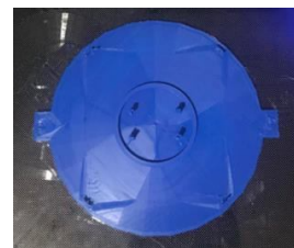
Fig. 2. The master model of the lower cover with new fastening elements is made
