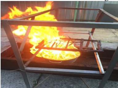
Figure 1 – An experimental installation for testing copper wires with an open flame
