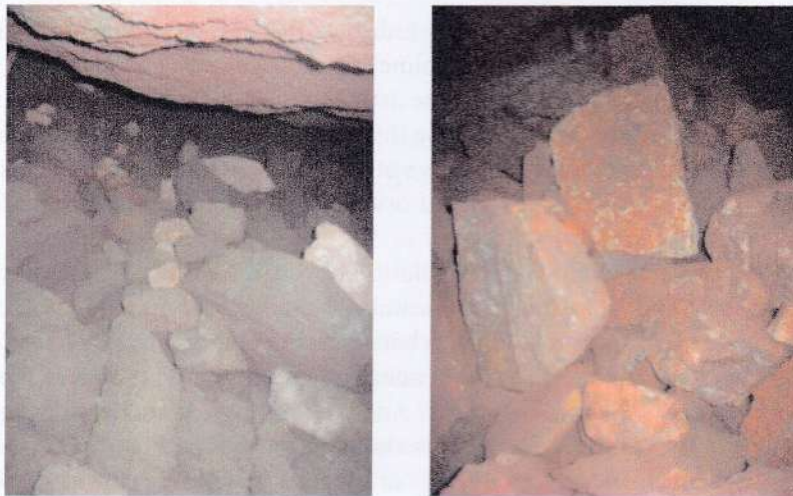
Fig. 12. Dilution of ore with backfill material when ore is mined from the stope
