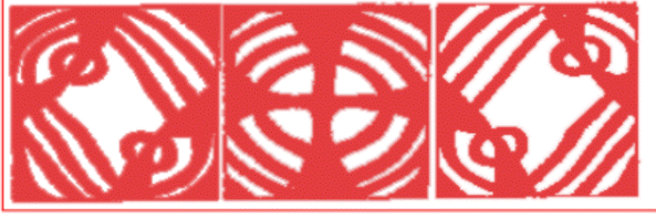
Fig. 3. View of the conoscopic figures of the \text{Rb}_2\text{SO}_4 crystal: (a) for the case T > 85 K (approaching OIP); (b) near OIP ( T = 85 K); (c) for the case T < 85 K (distance from OIP).
