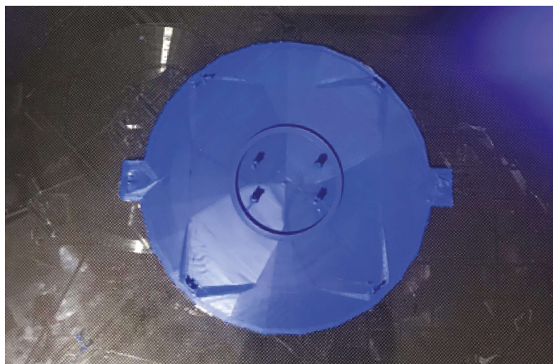
FIG. 3. The result of 3D printing of the FD lower cover body with new fastening elements
