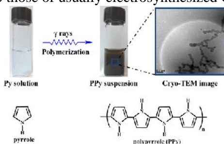
Fig 1. PPy synthesized by radiolytic method and in-situ observation of its morphology
