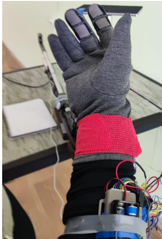
Figure 1. Smart glove connected to data acquisition unit
