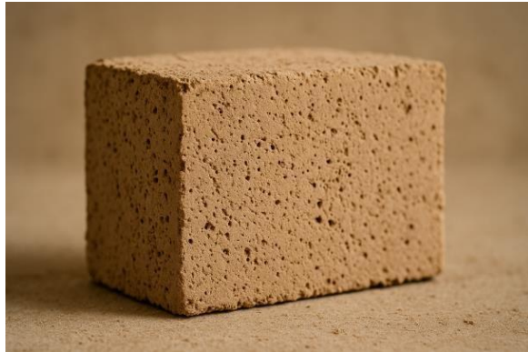
Fig. 1: Geopolymer concrete based on clay
