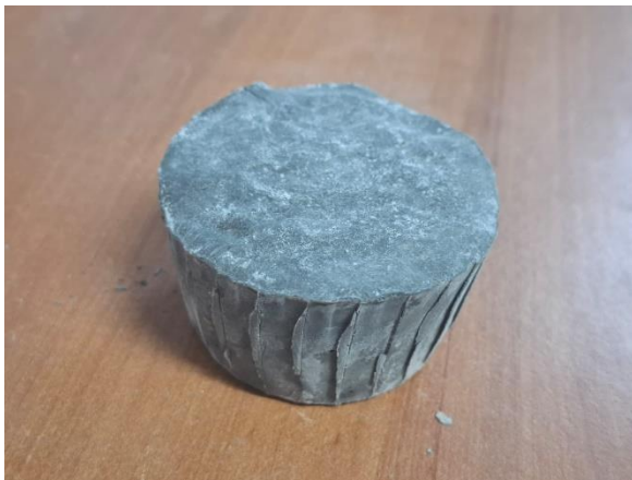
Fig. 1: Geopolymer concrete based on fly ash
