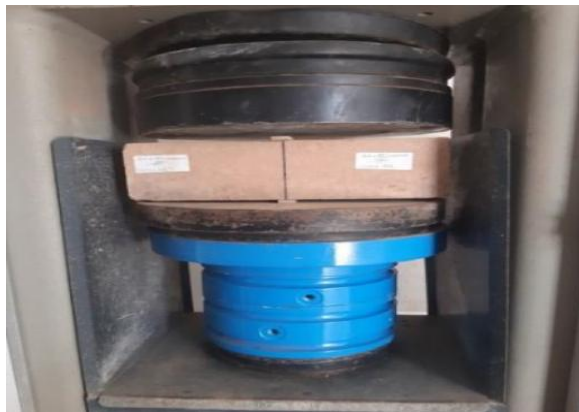
Fig. 1: Splitting tensile test (CDE, 2000)
