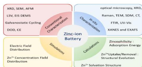
Fig. 1: Characterization, simulation, and calculation approaches for understanding zinc-ion batteries.
