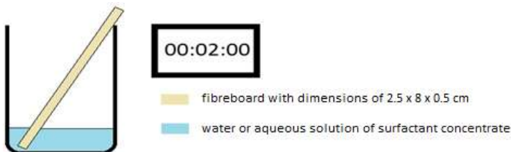
Picture 1. A scheme of an examination site for the saturation of the fibreboard samples
