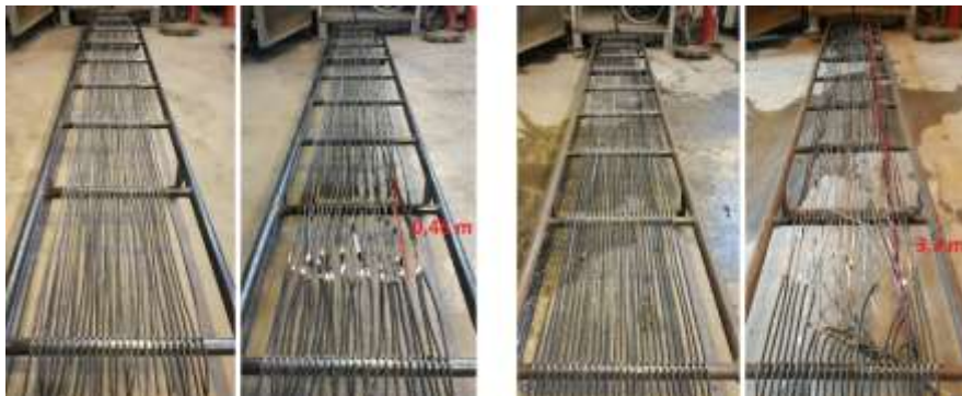
Photo 1. Cables before and after tests according to EN 50399 (on left cable H07Z1-R 1x10 with core class 2, on right H07Z-K 1x10 core class 5), Source: own materials
