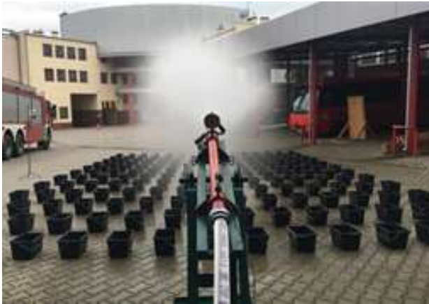
Draw. 2. TurboMaster nozzle during the research.
