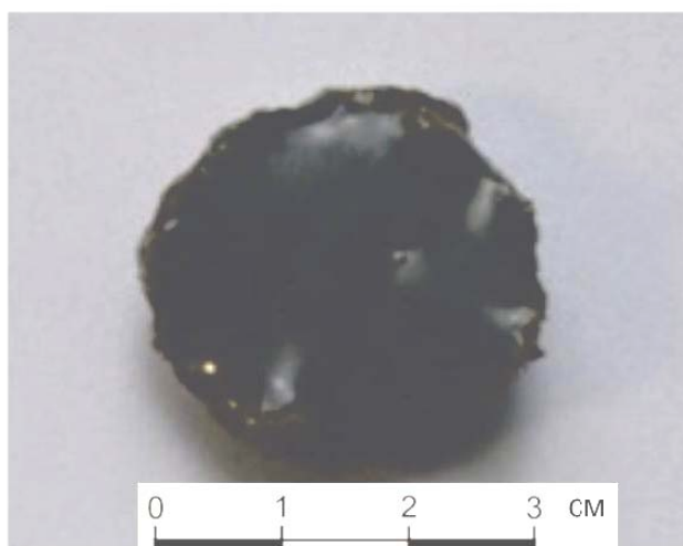
Figure 2 – Photo illustration of the product of firing clay loam (lower the horizon, the village of Ungurtas). The temperature-temporal parameters of firing stone material in a high temperature heating to 1200^{\circ}\text{C} (5', 40', 30')
