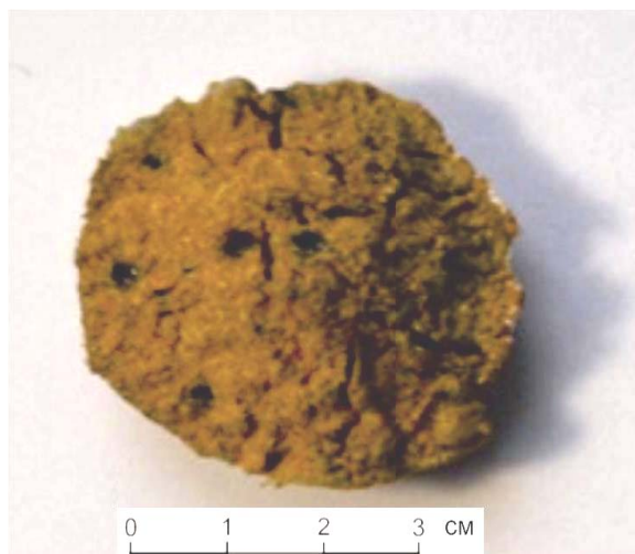
Figure 4 – Photo illustration (4) the product of annealing of the sample (the remains of an old storage pit Boraldai TPP); thermal-temporal parameters of firing stone material in a high temperature heating to 1200°C (5', 40', 30')
