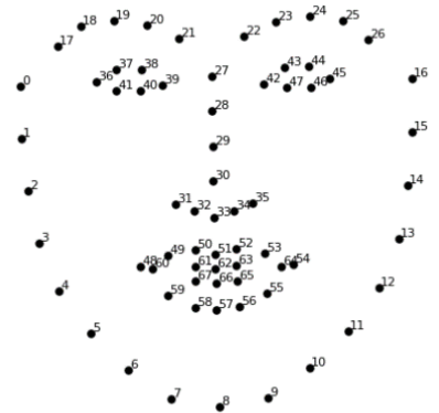
Fig. 2. All 68 points of reference, which will recognize the algorithm on the face.
