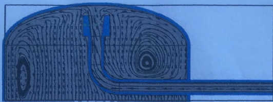
Fig. 7. Trajectories of gas motion inside the body of a discharge nozzle damping attachment
