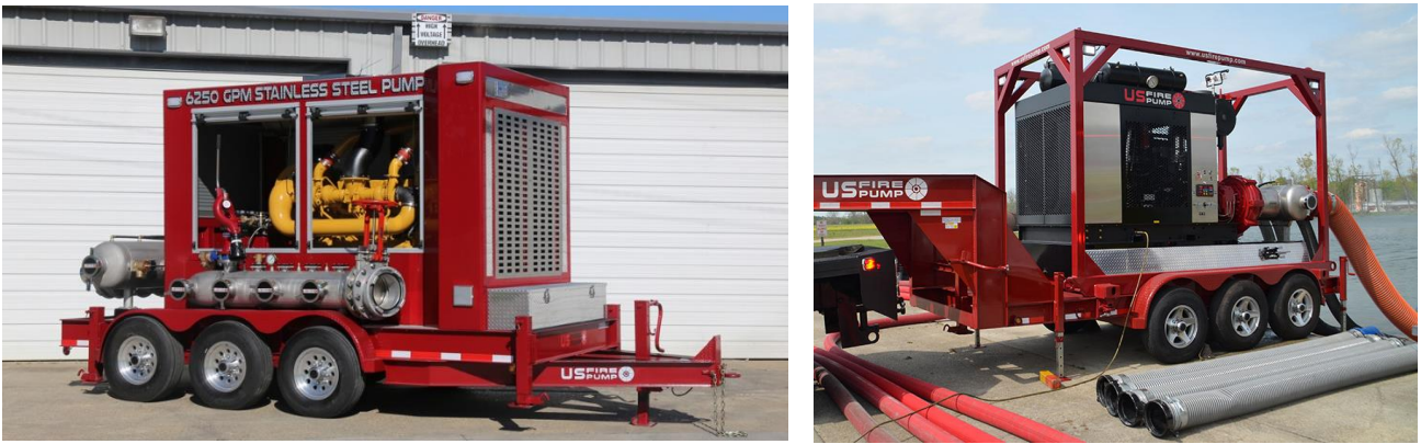
Figure 1. Mobile Pumping Station
