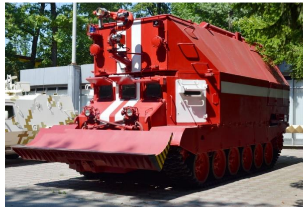
b) Special fire tank
