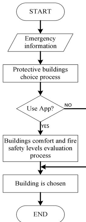
Fig. 6. The flowchart of protective building choosing process
