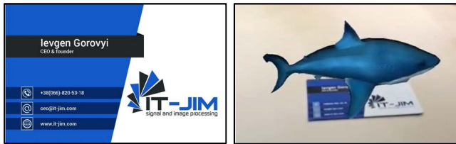
Fig. 4. Example of 3D model augmentation: image marker (left), 3D model over the detected marker (right)
