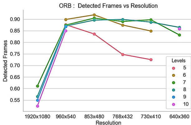
Fig. 10. Accuracy provided by ORB and AKAZE dependence on input image resolution and a number of levels.
