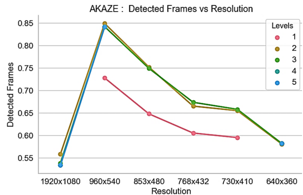
Fig. 10. Accuracy provided by ORB and AKAZE dependence on input image resolution and a number of levels.
