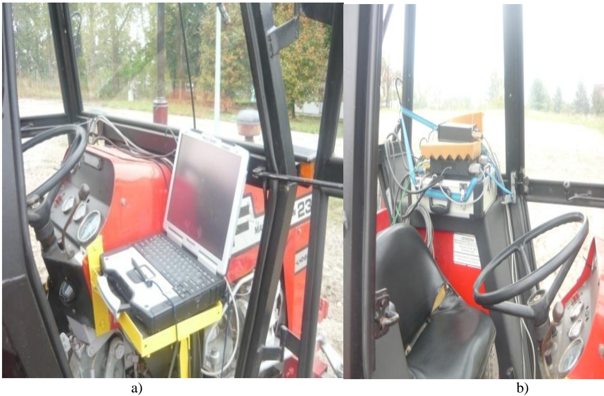
Figure 3. Measuring stand in the MF 235 tractor equipped with a) Panasonic CF 29 computer board and b) DaqBook 2000A measuring card
