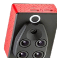
Fig. 3. The Sequoia multispectral chamber Source: Parrot Bluegrass Fields Drone [9].
